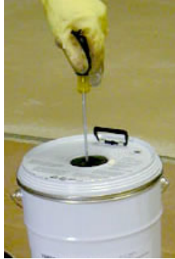
2. Pierce a hole through the top (rubber membrane) and the bottom of Part B container.
